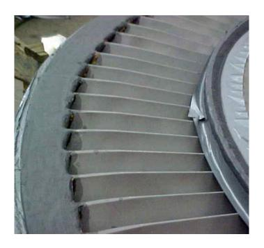
Belzona 1511 (Super HT-Metal) is a high temperature, paste-grade system for rebuilding equipment damaged by erosion-corrosion. This material can also be used as a high-strength structural adhesive or for the creation of irregular load bearing shims.
