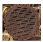
Heat exchanger tube face damaged by severe galvanic and pitting corrosion. Rebuilt with Belzona 1511 prior to the application of a Belzona high temperature coating.
